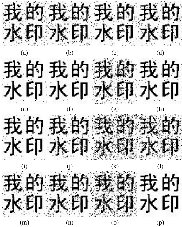
FIGURE 11. The extracted watermark image 1 for Lena image under different attacks: (a) Gaussian noise (0.05), (b) Gaussian noise (0.15), (c) Salt and Peppers noise(0.1), (d) Salt and Peppers noise (0.2), (e) Median filtering (5 × 5), (f) Wiener filtering (5 × 5), (g) JPEG compression(5%), (h) JPEG compression (20%), (i) Scaling (1/8), (j) Cropping (center 128 × 128), (k) Cropping (Edge 64 × 512), (l) Translation (5 pixels), (m) Rotation (5°), (n) Rotation (10°), (o) Rotation(40°), (p) Rotation (90°).
