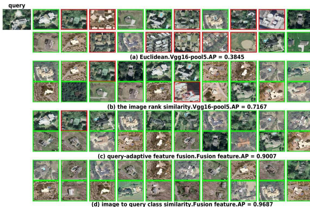
FIGURE 5. Retrieval results comparison in each step. The first column is the query image from UCMD, (a) the top 20 result of Vgg16-pool5 using Euclidean, (b) the top 20 results of Vgg16-pool5 using the image rank similarity, (c) the top 20 results of four features by the query-adaptive feature fusion, (d) the top 20 results of fusion feature using the image to query class similarity.
