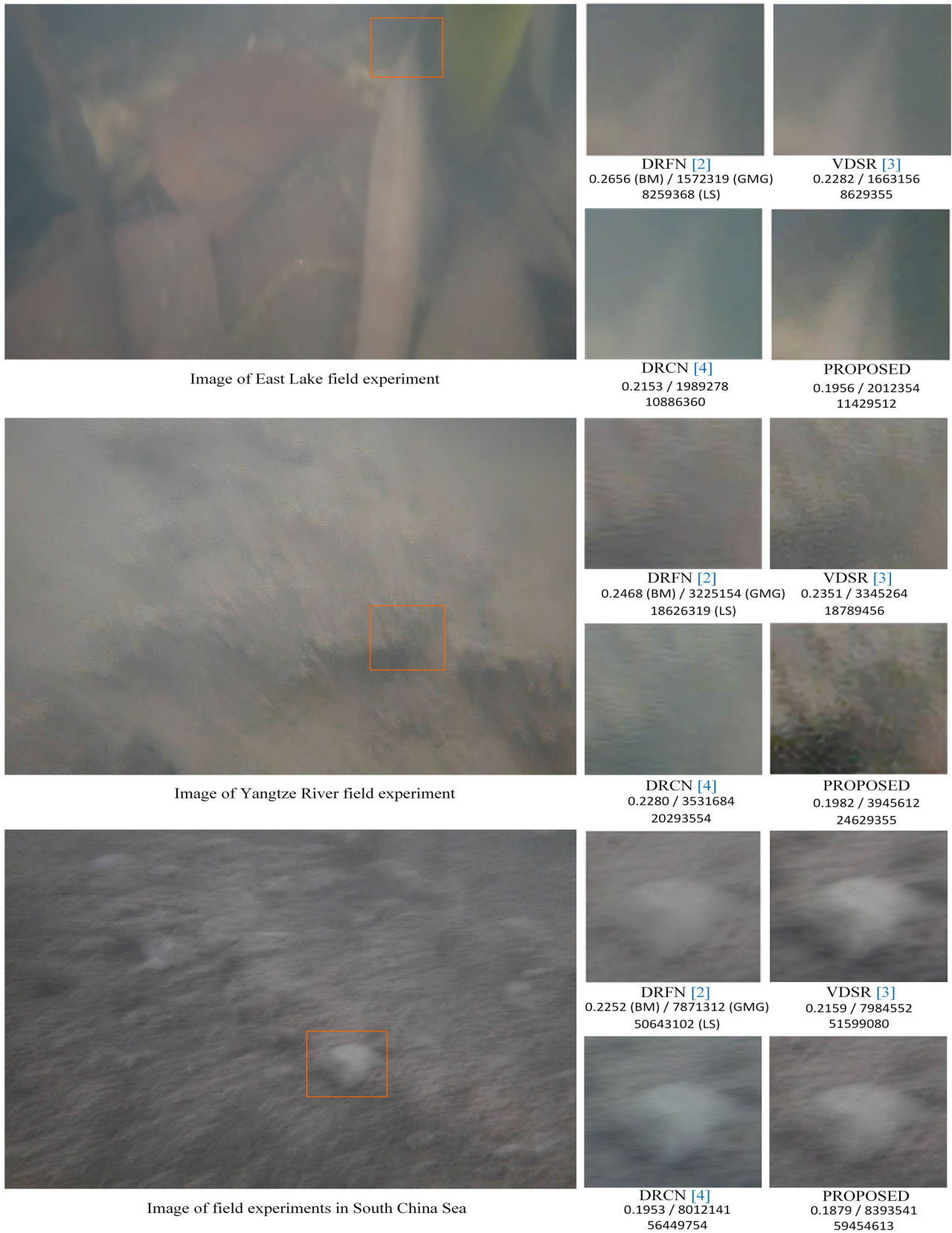
FIGURE 10. Super-resolution result of our method compared with existing algorithms in field experiment.
