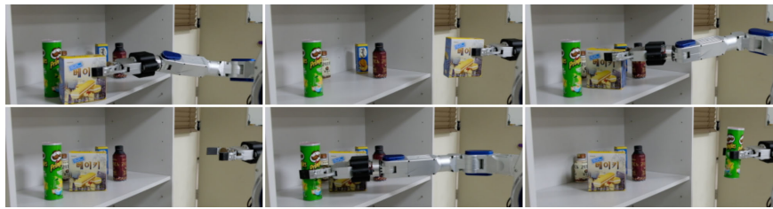
(a) M-Hubo relocates the yellow cookie box to an empty space and grasps the target item.
