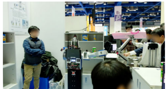
FIGURE 20. A snapshot of the public demonstration in an exhibition hall. The arrangement of the furniture was the same with the lab setting whereas their coordinates were slightly different. Several environmental conditions were unfavorable: carpeted floor incurring slips, poor lighting condition, and no wired power supplies for the bearbone computers and the robot actuators.
