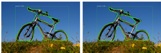
FIGURE 1. When the complexity of the image structure is normal, the segmentation results of the smaller bounding box on the left and the larger bounding box on the right are almost the same.
