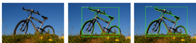
FIGURE 3. Visual comparison of Mask R-CNN using traditional NMS and Syncretic-NMS. From left to right are the original image, the prediction result that was obtained using traditional NMS, and the prediction result that was obtained using Syncretic-NMS. Syncretic-NMS can effectively improve the prediction result, the bounding boxes can more completely contain the entire object, and the objects that are outside the bounding box can now be correctly predicted.
