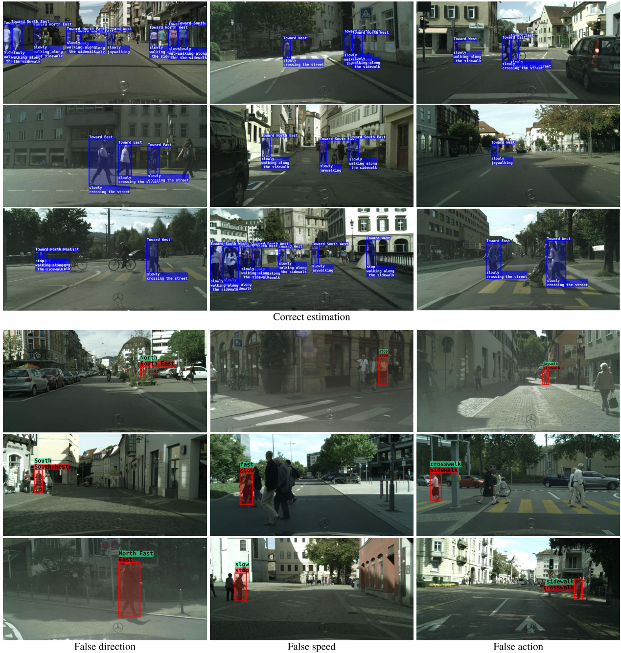
FIGURE 9. FM estimation results of CityPersons data in the FM dataset. The top three rows present correct estimation results. The bottom three rows show failure cases, where green and red labels are the ground-truth and predicted classes, respectively.
