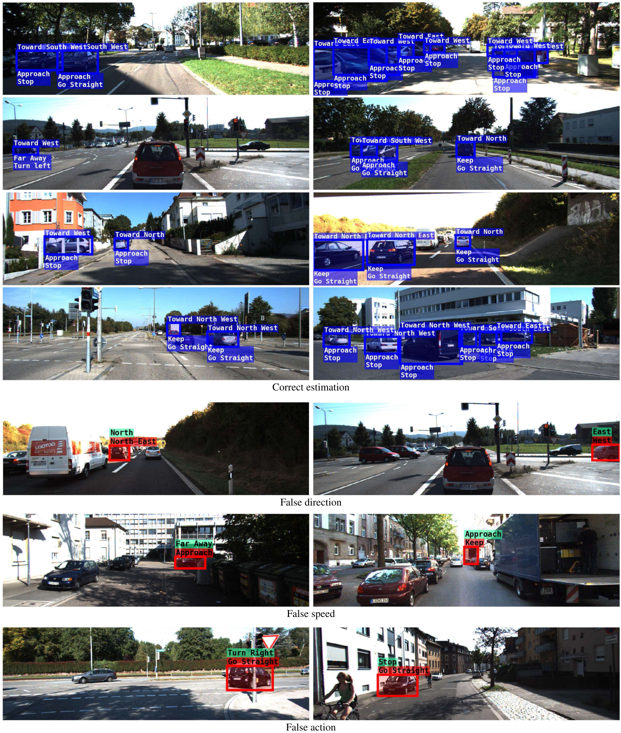
FIGURE 11. FM estimation results of car instances. The top four rows show correct results. The bottom three rows are failure cases, where green labels are the ground-truth and red labels are predicted classes.
