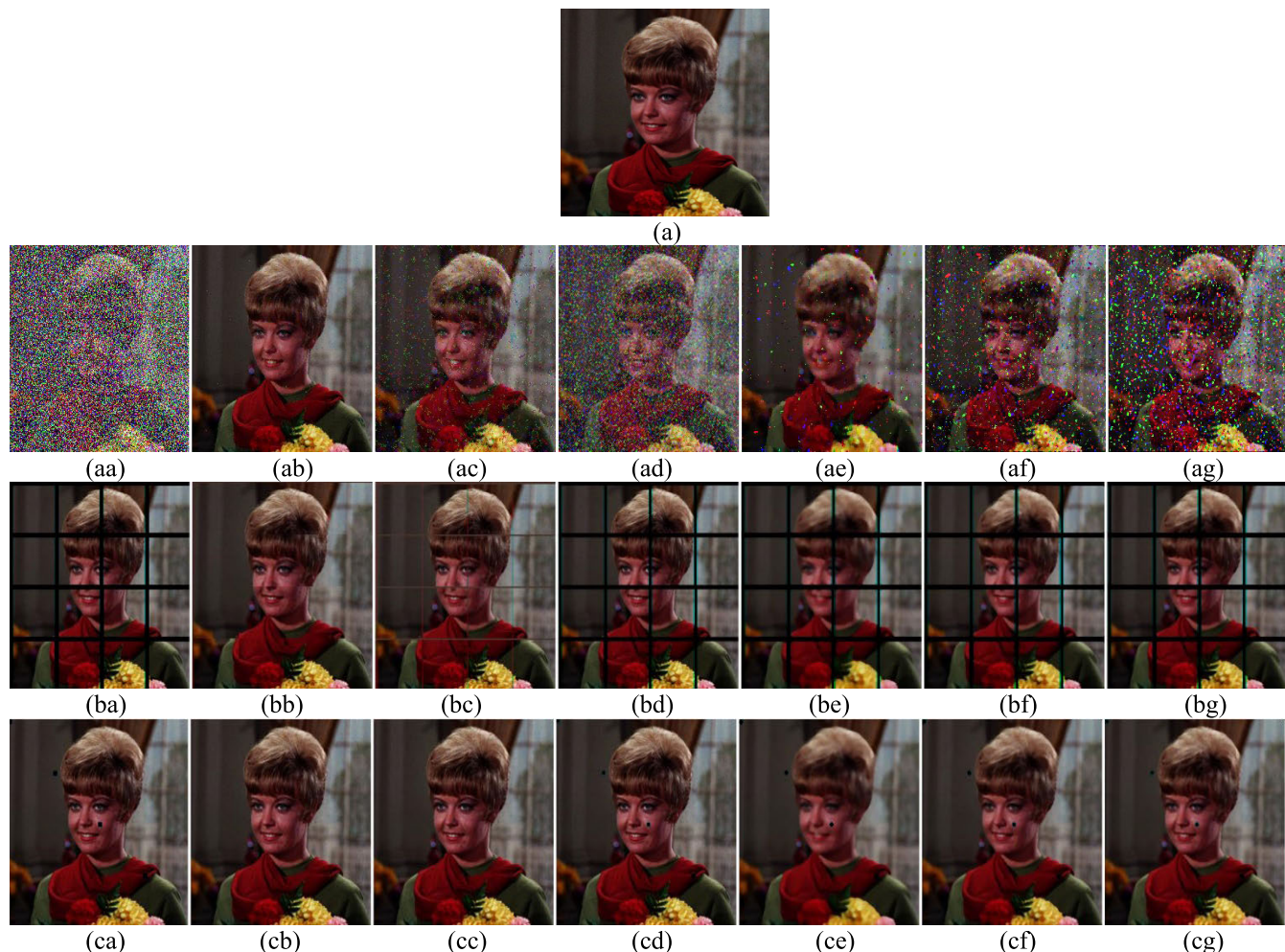
FIGURE 17. (a) Original color image, (aa) Color image corrupted by 50% Salt and Pepper noise, (ba) Color image corrupted by 6 pixel wide strip line artifact, (ca) Color image corrupted by 6 * 6 pixel size blotches artifacts, (ab–cb) Image restored using proposed method from (aa–ca), (ac–cc) Image restored using the ROAD-TGM from (aa–ca), (ad–cd) Image restored using the DBMF from (aa–ca), (ae–ce) Image restored using the CWMF from (aa–ca), (af–cf) Image restored using the PSMF from (aa–ca), (ag–cg) Image restored using the MF from (aa–ca). NB: ROAD-TGM, Rank-Ordered Absolute Differences Trimmed Global Mean Filter; CWMF, Center Weighted Median Filter; DBMF, Decision-Based Median Filter; PSMF, Progressive Switching Median Filter; and MF, Median filter.
