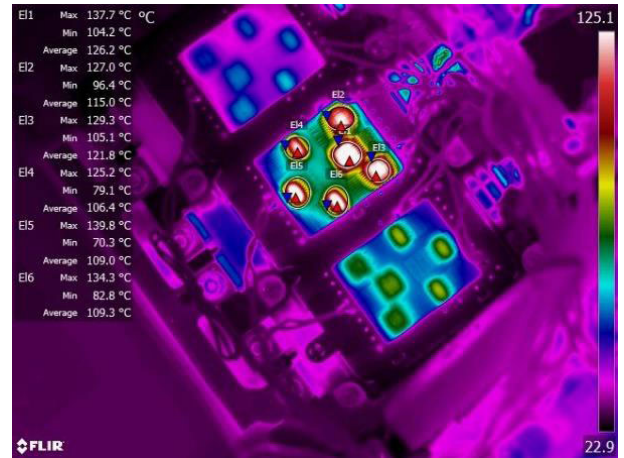
FIGURE 14. The results of thermal infrared camera under the 550A locked-rotor current.
