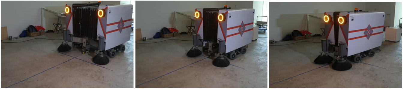
FIGURE 18. Reconfiguration in width during locomotion.
