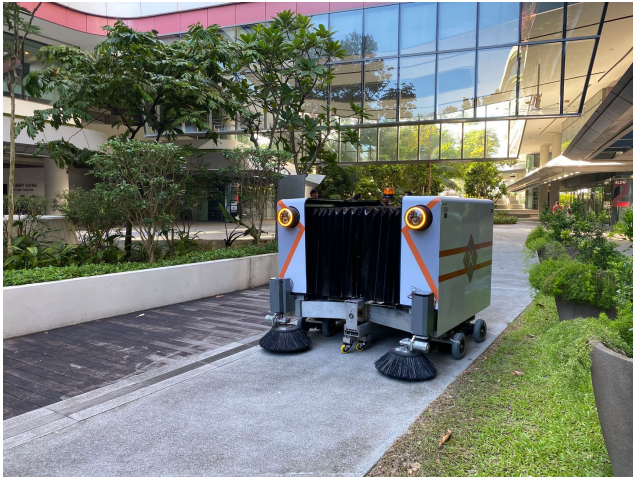
FIGURE 1. Panthera: Reconfigurable pavement sweeping robot.
