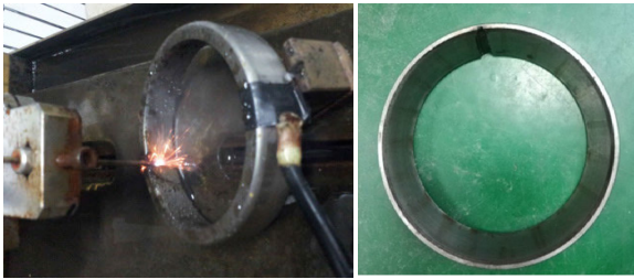
FIGURE 13. Electric discharge machined bearing outer ring.
