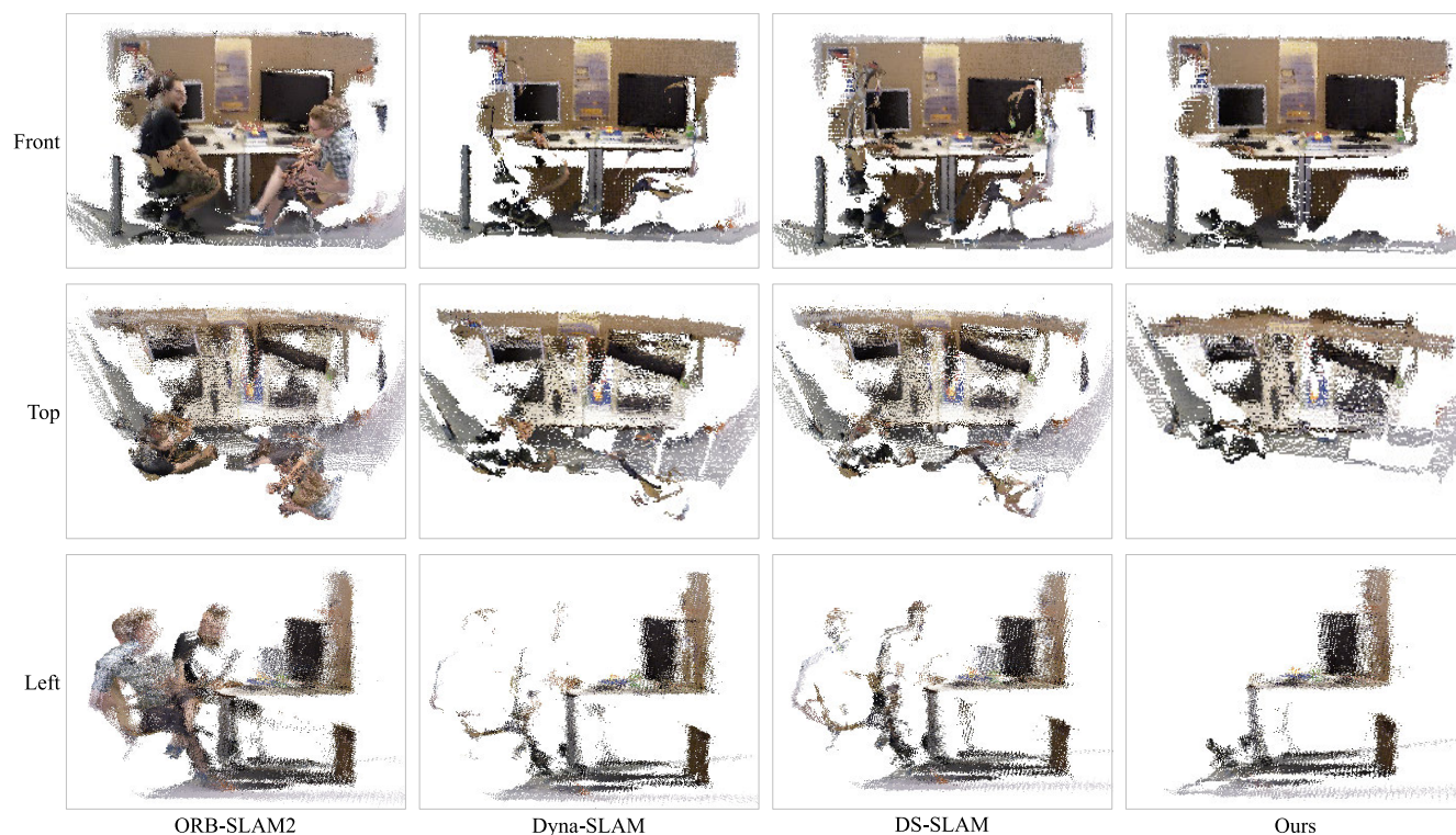
FIGURE 16. Comparison of global point cloud maps constructed by the four SLAM systems on fr3/s/static.
