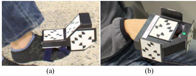
FIGURE 4. Markers to measure the position and posture by a motion capture camera. (a) Marker equipment mounted on foot. (b) Marker equipment mounted on hand.
