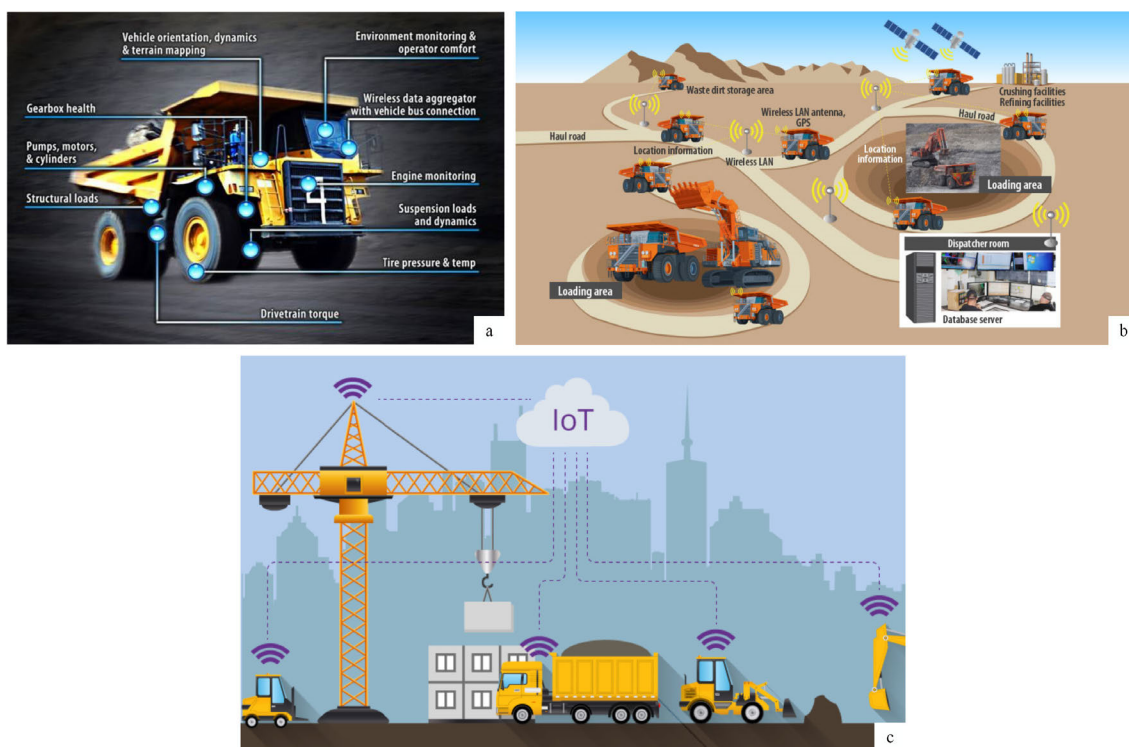
FIGURE 2. The applications of sensor technologies for construction machinery: (a) Condition monitoring [3]; (b) Autonomous construction [4]; (c) IoT [5].
