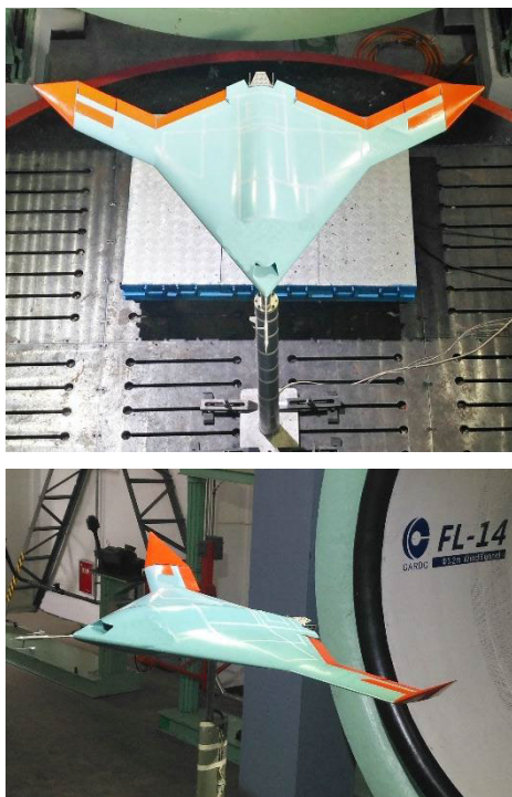
FIGURE 2. Tailless aircraft model on the 3-DOF dynamic rig.
