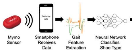
FIGURE 3. Flow of Mymo system from wearable to shoe classification.
