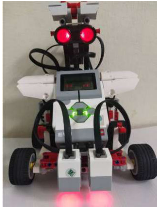
FIGURE 1. PvBOT - a LEGO Mindstorms EV3 robot for teaching place values.
