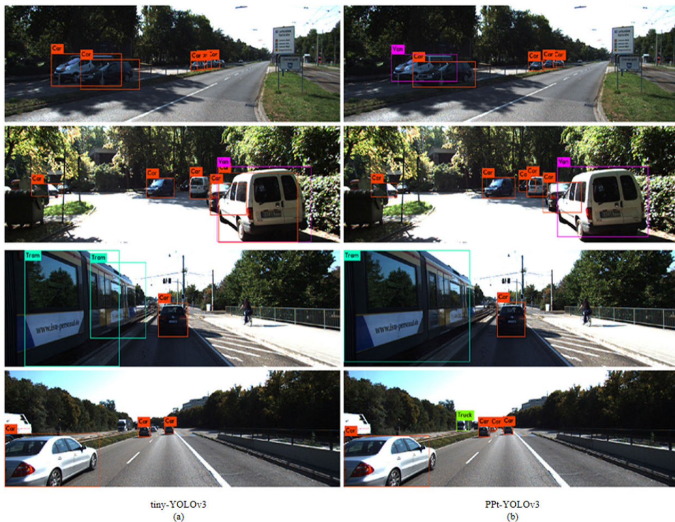
FIGURE 7. The comparison of detection results of images in KITTI dataset with tiny-YOLOv3 and PPt-YOLOv3. Four pictures on the left were detected with tiny-YOLOv3, and four pictures on the right were detected with PPt-YOLOv3. A group of horizontal pictures are the same scene.
