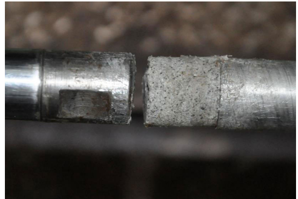
FIGURE 2. The fracture surface of a specimen under specimen unreinforcement.
