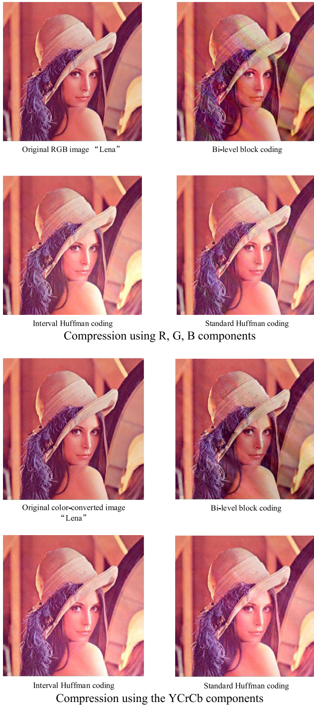
FIGURE 7. Comparison results using predictive 2-D bi-level block coding, predictive interval Huffman coding and predictive Huffman coding at BER = 0.005 for "Lena" image.
