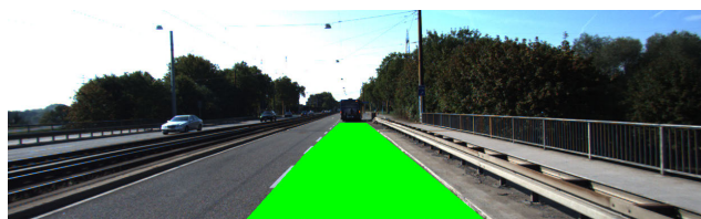
FIGURE 1. A typical ego-lane detection result in the KITTI Lane dataset, where the ego-lane is labeled as green.
