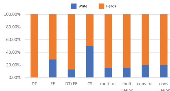
FIGURE 10. Normalized ratio of reads and write in the memory for the considered edge-level applications.
