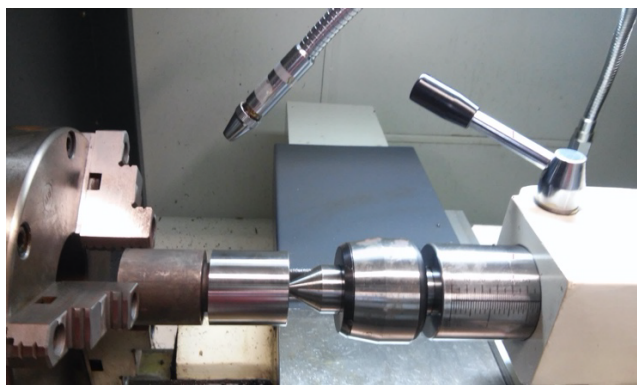
FIGURE 2. Turning operation of AISI 52100 hardened steel.
