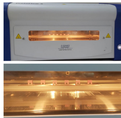
FIGURE 9. Ridge ceramic blocks soldered with bottom lid first using LPKF reflow oven.
