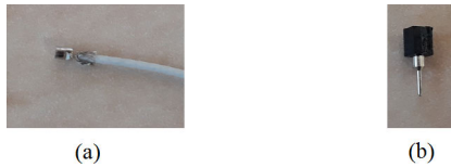
FIGURE 7. Used electric dipoles (a) for modeling neural activity and electrode pins (b) for monitoring surface electric potential.
