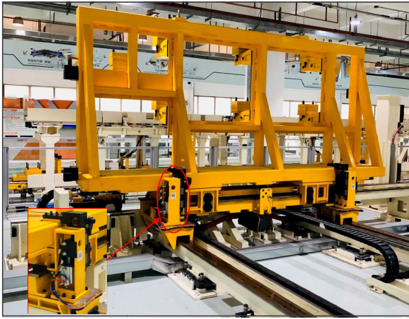
FIGURE 3. The data collecting site with a cylinder on the trolley.
