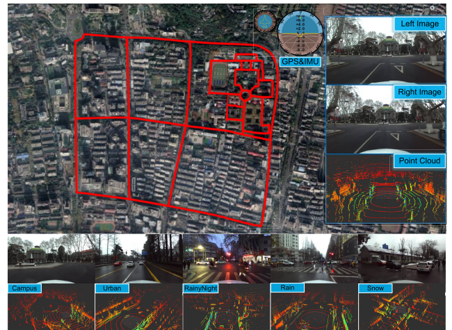
FIGURE 5. Demonstration of our dataset. We collect data on the same path of campus and city roads under different times and weather conditions, including binocular images, LIDAR point cloud, GPS, and IMU data, with a total length of nearly 50 kilometers.
