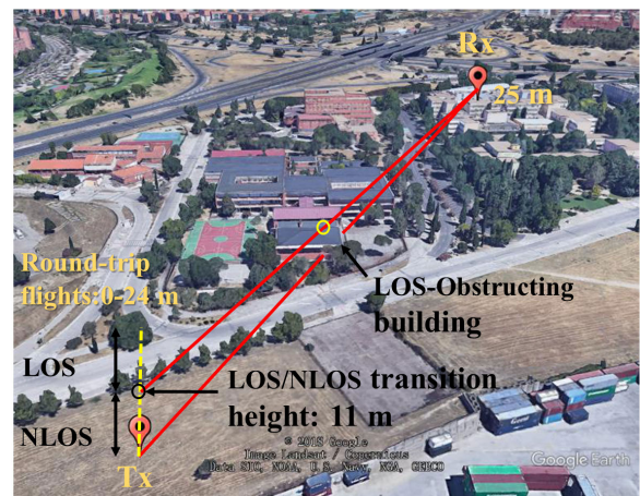
FIGURE 2. Measurement environment and setup where the altitude of the UAV-integrated Tx is 0-24 m (round-trip flights) and the Rx height is 25 m.
