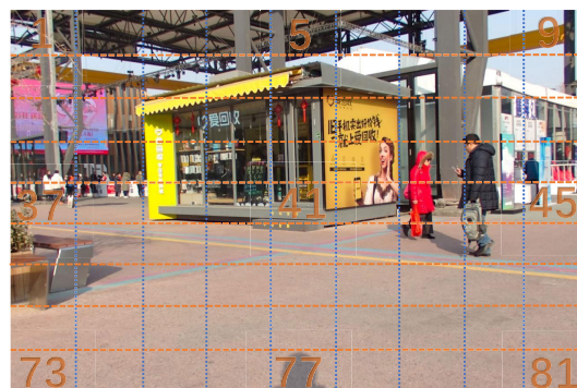
FIGURE 3. Considering the proportion of individual pedestrian pixels in the whole image, we divide rows and columns into 9 parts on average and get 81 regions, as shown by the dash lines in the figure.
