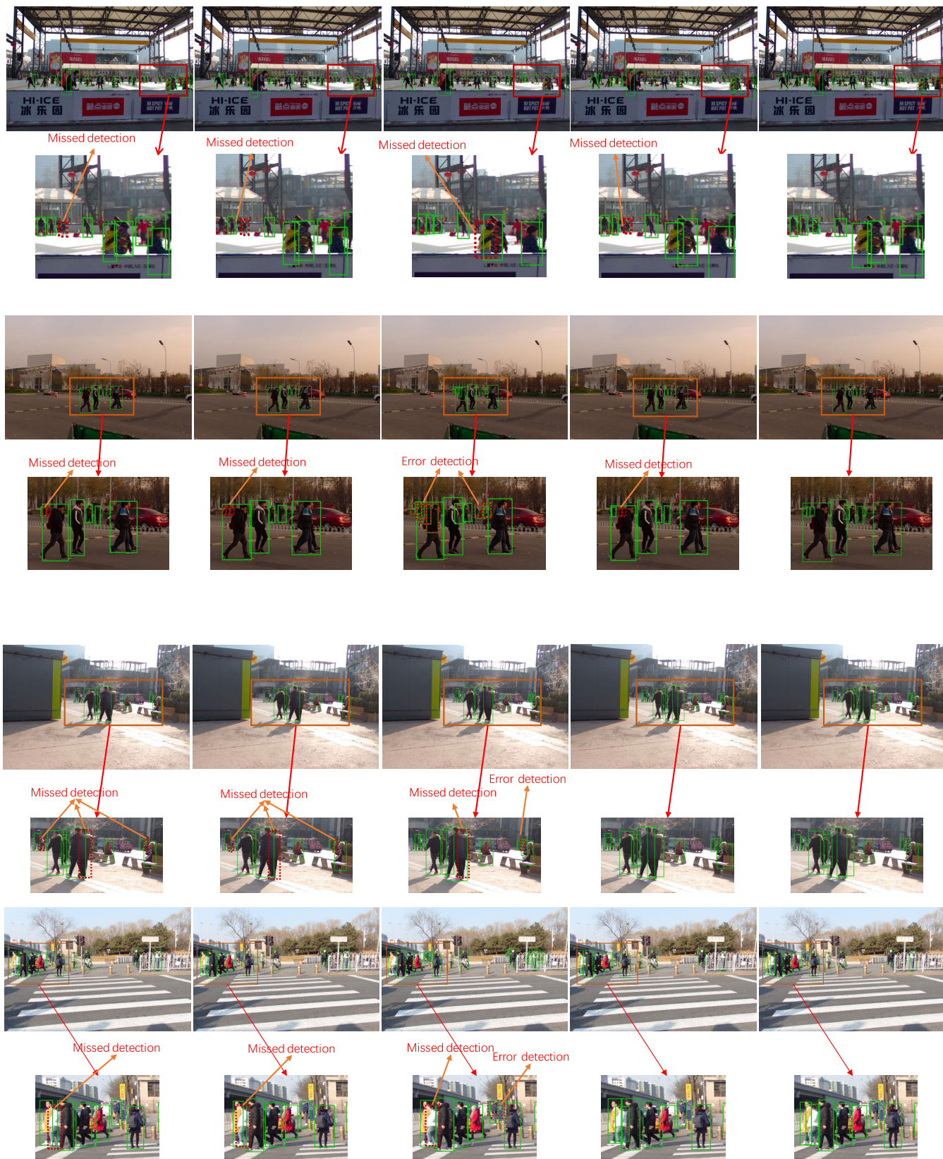
FIGURE 7. Comparisons with state-of-the-art methods. (From left to right) ALFNet, CSPNet, Faster-RCNN, Reploss, and Ours. The green rectangle represents the detection results and the red rectangle represents missed detection and error detection.
