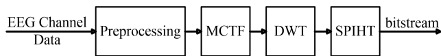
FIGURE 1. Block diagram of the proposed motion compensated temporal filtering based EEG compression encoder.
