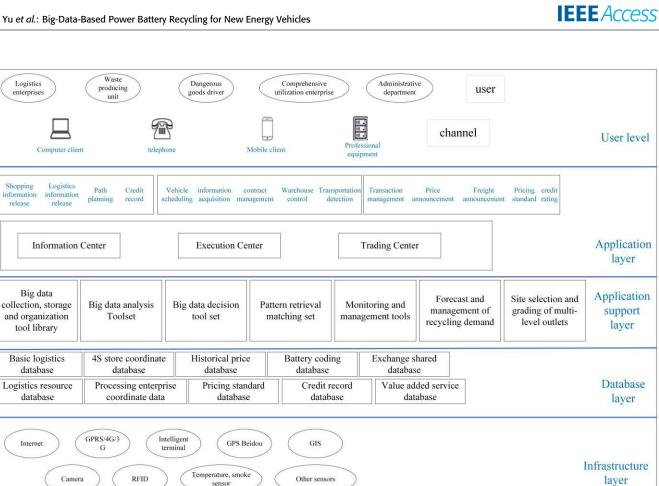
FIGURE 2. Theoretical model of a power battery recovery platform based on big data.
