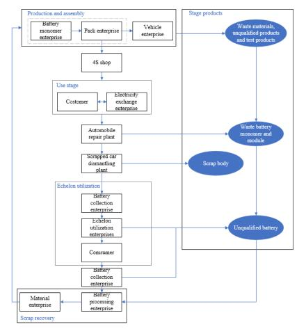
FIGURE 1. Power battery life cycle recovery pipeline process.
