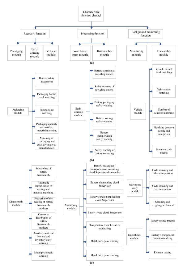
FIGURE 4. Logic structure model of characteristic function pipeline of power battery recovery platform based on big data.
