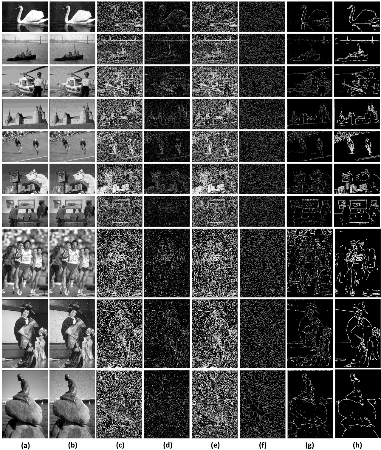
FIGURE 8. Noise-containing image edge detection results. (a) Original image, (b) ground truth by human subjects, (c) edge produced by RONG+Canny, (d) edge produced by WAN+GM (1,1), (e) edge produced by LI+GRA, (f) edge produced by ZHENG+Morphology, (g) edge produced by PENG+Moment, (h) edge produced by proposed algorithm.
