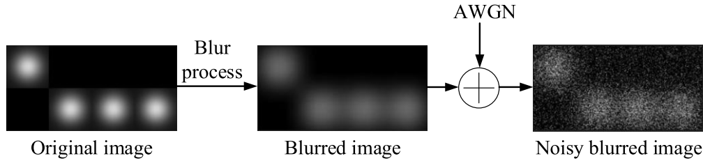
FIGURE 3. Channel model in vehicular OCC system.
