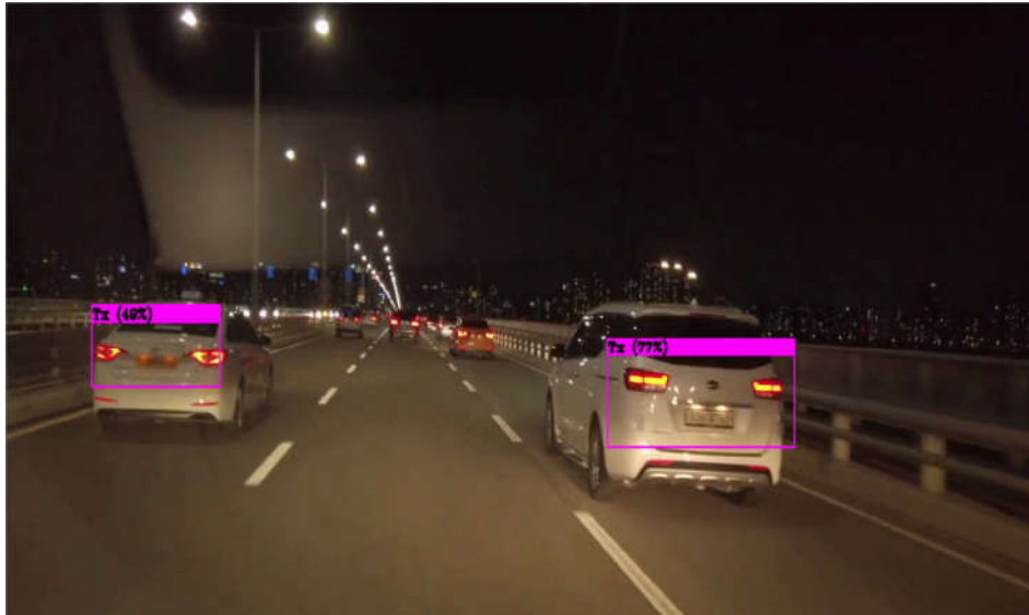
FIGURE 15. A test on using YOLOv2 for city driving inside Seoul at night.
