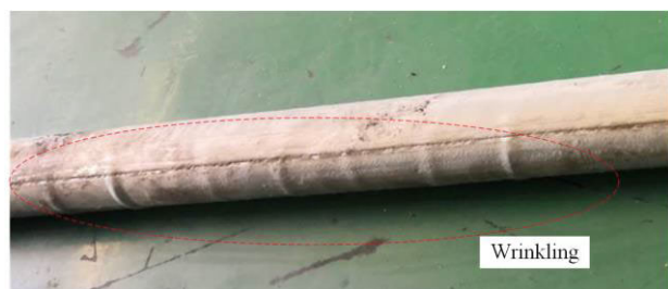
FIGURE 4. Wrinkling of the smooth aluminum sheath unbonded.
