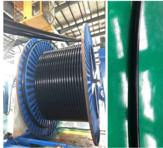
FIGURE 8. The 110 kV XLPE cable with smooth aluminum bonded sheath.
