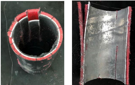
FIGURE 7. Interface delamination of Sample B after aging.
