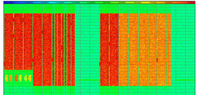
FIGURE 20. The power per RE versus the subcarriers (vertical axis) and the OFDM symbols (horizontal axis) in case of one UE in A and one UE in B and full use of the grid resources; the power level is plotted in false colors.
