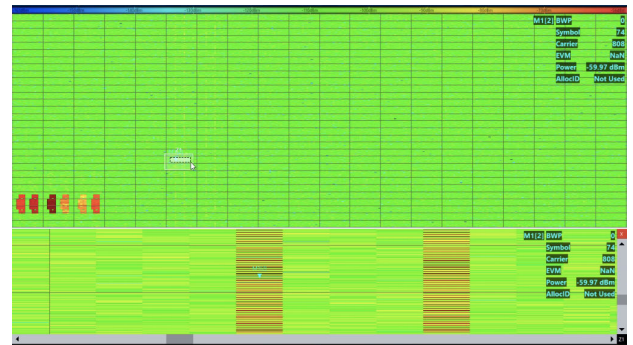
FIGURE 11. The figure shows the power per RE versus the subcarriers (vertical axis) and the OFDM symbols (horizontal axis) in a frame in case of no traffic data; the power is represented in false colors; the brightest red is -45 \text{ dBm} ; the upper part of the figure shows the entire RG; the lower part shows a zoom of the area of the grid indicated by the bright rectangle in the upper figure.
