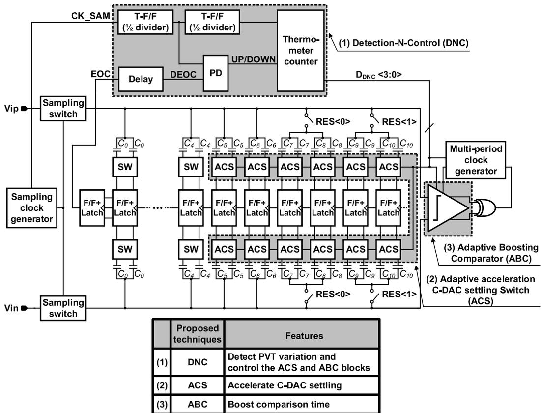
FIGURE 5. Block diagram of proposed ADC.
