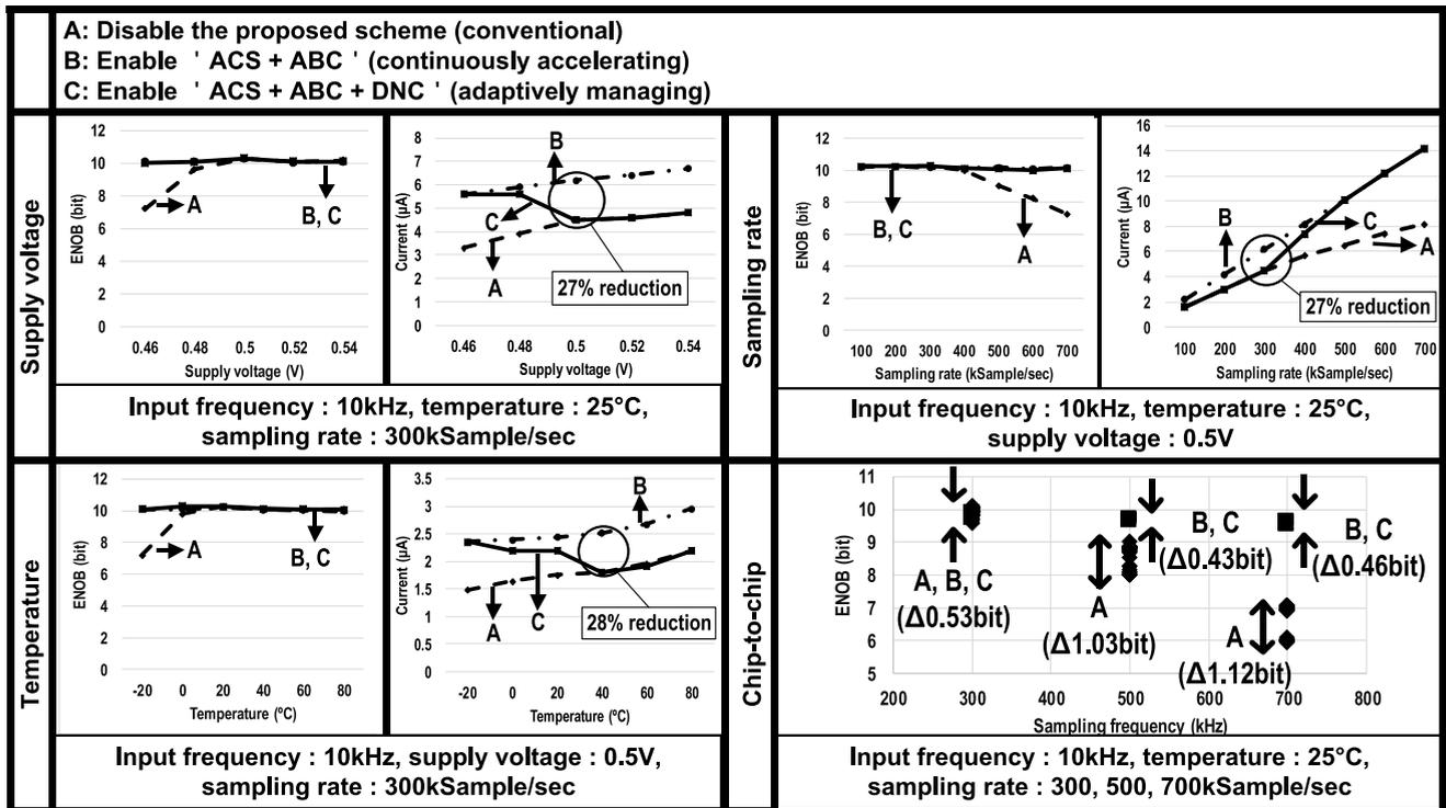
**FIGURE 11.** The measured ENOB and current (power consumption). In this figure, A, B, and C indicate 'disable the proposed scheme (conventional)', 'enable (ACS + ABC)', and 'enable (ACS + ABC + DNC)'.
