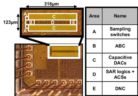
FIGURE 10. Fabricated die micrograph.
