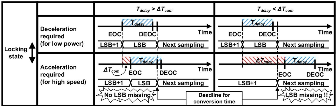
FIGURE 4. A locking state and criteria to prevent the least-significant-bit (LSB) missing.
