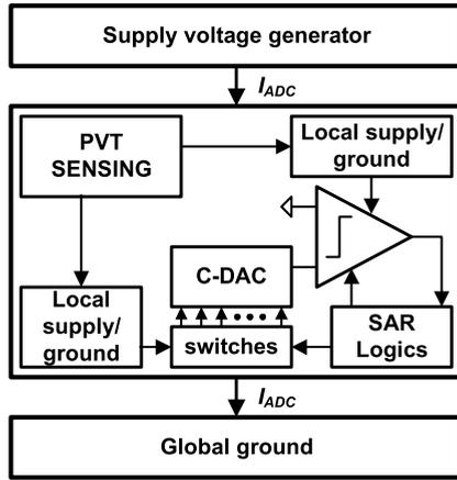
FIGURE 3. The conceptual block diagram of the proposed PVT compensation system.
