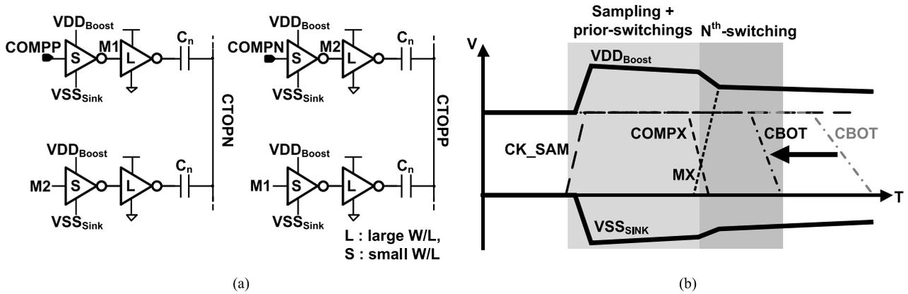
FIGURE 7. The (a) implementation of adaptive acceleration C-DAC settling switch (ACS) and (b) effect of capacitive digital-to-analog converter (C-DAC) acceleration.
