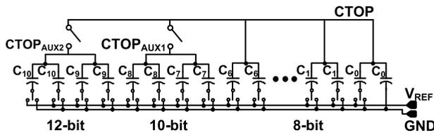
FIGURE 9. Schematic of C-DAC with resolution reconfigurable function.
