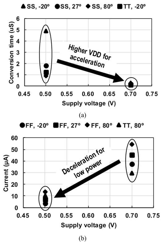
FIGURE 2. (a) The process, voltage, and temperature (PVT) conditions that require acceleration by increasing VDD (supply voltage) and (b) the other PVT conditions that can reduce the current for low power operation.
