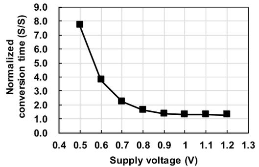
FIGURE 1. Normalized conversion time at the worst-case corner and temperature conditions with various supply voltages from 0.5 V to 1.2 V.
