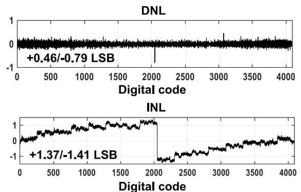
**FIGURE 13.** The measurement results of static performance.
