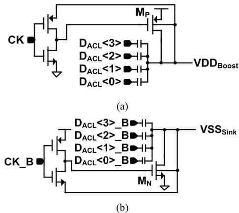
FIGURE 6. Schematic of (a) VDD-Booster and (b) VSS-Sinker for local supply/ground voltages.
