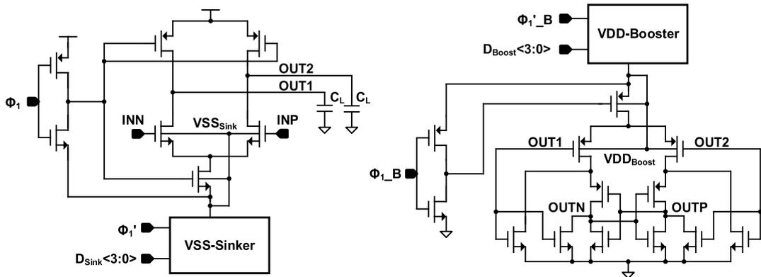
FIGURE 8. The schematic of an adaptive boosting comparator (ABC).
