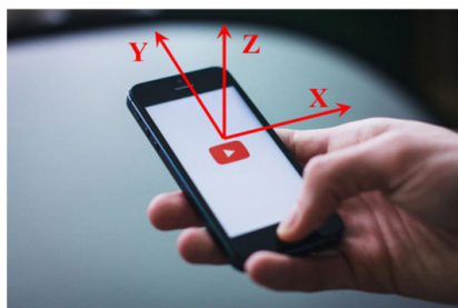
FIGURE 3. The coordinate system of the smartphone used in this study.
