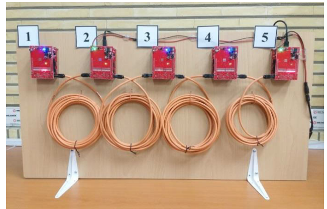
FIGURE 19. A simple setup for qualifying the performance of the proposed fail-over mechanism.
