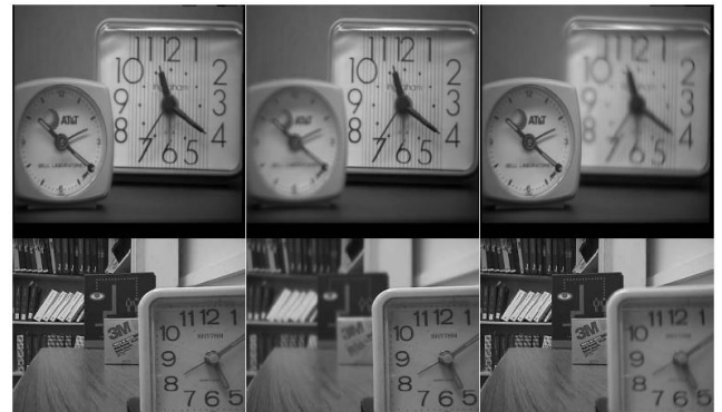
FIGURE 6. Two gray test images 'clock' and 'disk'. The first column are ground-truth reference images (focus everywhere); The second and third columns are source images with focus on right and left respectively.
