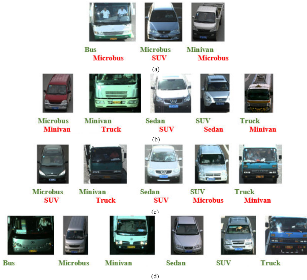
FIGURE 9. Examples from the classification results of BIT-RXD and BIT-XD for vehicle images that are (a) Correctly classified by BIT-RXD and misclassified by BIT-XD (b) Correctly classified by BIT-XD and misclassified by BIT-RXD (c) Incorrectly classified by both super learners (d) Correctly classified by both super learners (The Red caption is the ground truth, and the red caption indicates a misclassification).
