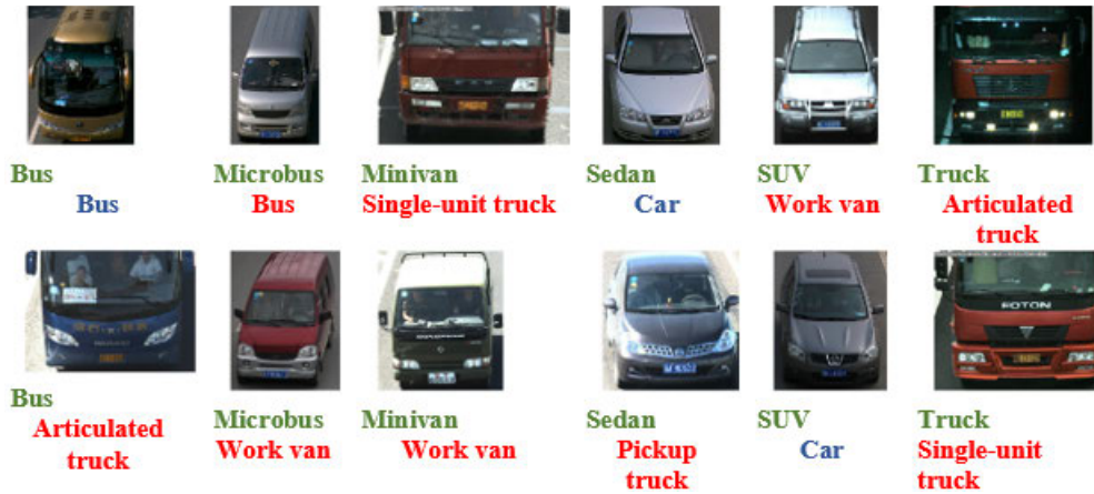
FIGURE 6. Examples of the classification results on the BIT-vehicle dataset (The green caption is the ground truth from the BIT-Vehicle dataset, the red caption is the predicted class from the MIO-TCD dataset, and the blue caption indicates a correct equivalent label).
