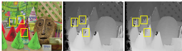
FIGURE 5. Qualitative result analysis between ours and original SGM for Cones dataset. Yellow boxes depict the improvements of our approach in discontinued regions. left: reference, middle: original SGM result, right: our result.
