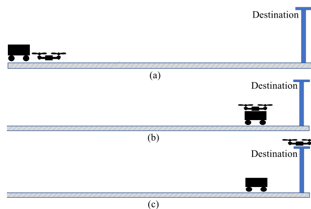
FIGURE 1. An example of a UGV-UAV complementary coalition for task completion: (a) the target destination is too far for the UAV to reach, while too high for the UGV alone, (b) the UGV carries the UAV closer to the destination, and, finally, (c) the UAV flies to the high-altitude destination.
