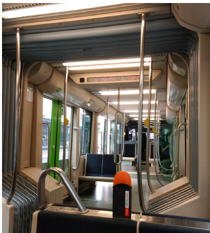
FIGURE 3. EME Spy Evolution personal dosimeter used in the campaign of measurement placed within the tram.
