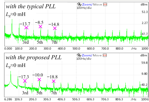
FIGURE 18. Grid current spectra with different PLLs and L_g \approx 0 obtained from the oscilloscope.
