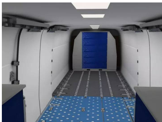
FIGURE 2. Inside of HEFTs with large middle doors on both sides and fastening tracks on the floor.
