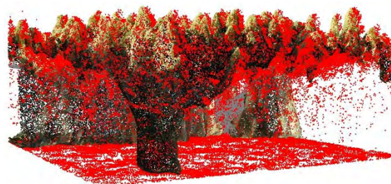
FIGURE 4. Display of point cloud registration results. The colored points represent the oblique photography point cloud, and the red points represent the LiDAR point cloud.
