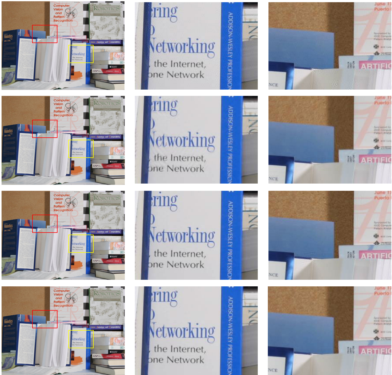
FIGURE 14. Results of watermarked center image of the proposed and comparative methods. From top to bottom, the results denote the watermarked images of the IR-based, DTCWT-based, SIFT-based, and proposed method, respectively. The second and third columns are the results of enlarging the areas of the yellow and red boxes of the image of each first column, respectively.
