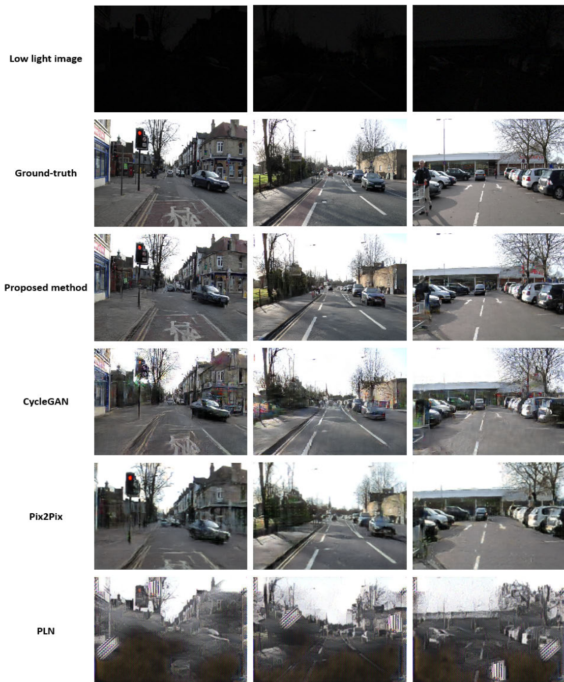
FIGURE 6. Examples of low light image enhancement results of the Syn-CamVid database. The first row shows the input images of the source domain, the second row shows each low light image and the accumulated ground-truth daytime images of the target domain, and the third row to the last row show the enhancement result images obtained by the proposed method, CycleGAN, Pix2Pix, and PLN, respectively.
