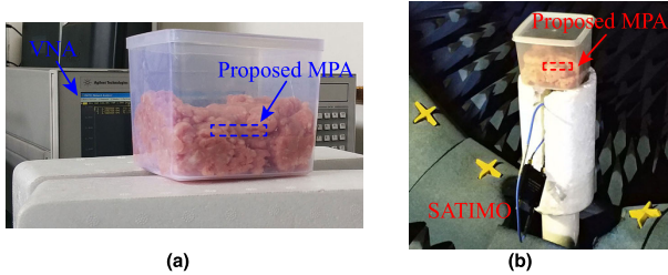
FIGURE 23. Photographs of experimental set-up for measuring the proposed MPA: (a) vector network analyzer, (b) SATIMO near-field antenna measurement system.
