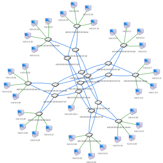
FIGURE 6. The simulated topology of the fattree.
