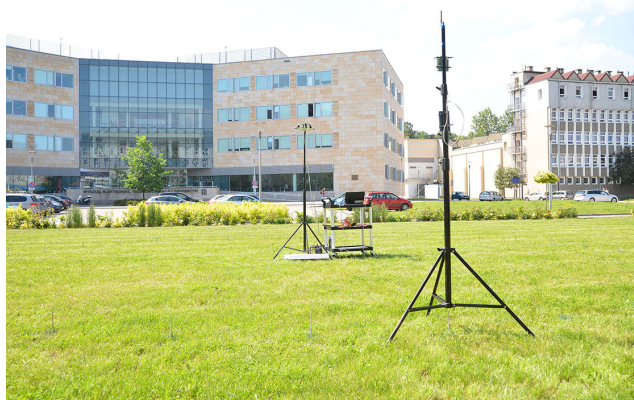
FIGURE 12. Test setup arranged for the measurements in 3 meters distance.
